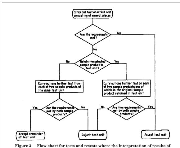
non-sequential tests is based on individual values only (e.g. for tensile tests) for cases where the test unit consists of several piece
